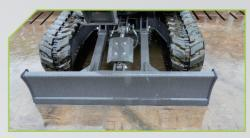
The dozer plumbing is equipped with a protective plate to cope with difficult working conditions, protecting the cylinder and line at the same time.
