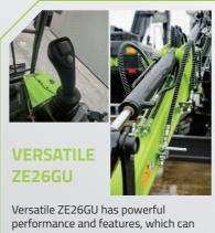
Versatile ZE26GU has powerful performance and features, which can easily meet customer needs. A high configuration model is equipped with a breaker plumbing, a quick coupler plumbing, and multiple attachment plumbings, and allows the user to control the plumbing with a switch on the joystick for easier operation.
